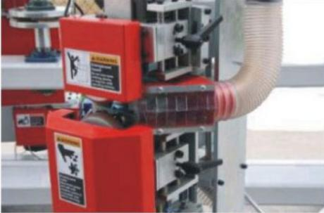
adjustment for boards of different thickness. The thickness is adjusted automatically by the machine.
