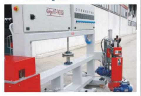
The trimming unit's operation is automatic and similar to that of banding unit's. The trimming unit is used for cleaning the overhangs at top and bottom sides of the board. The trimming unit is programmed for rotating the board and for the operation of the trimming motors. The guiders follow the board from the top, while the trimming unit cleans the overhangs of edges by adjusting its position according to the board edges.
