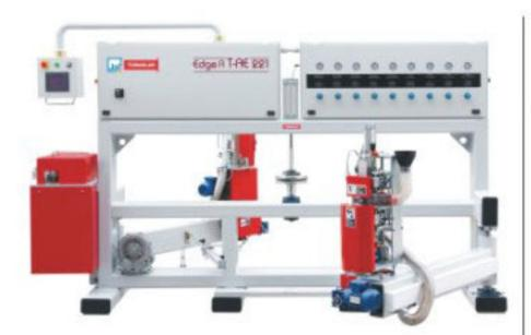
have been designed PLC based. With its multifunctional design, it operates much faster, when we compare it to manually operated machines, and it also provides high quality banding and trimming processes. Its use requires less effort for the operator.
