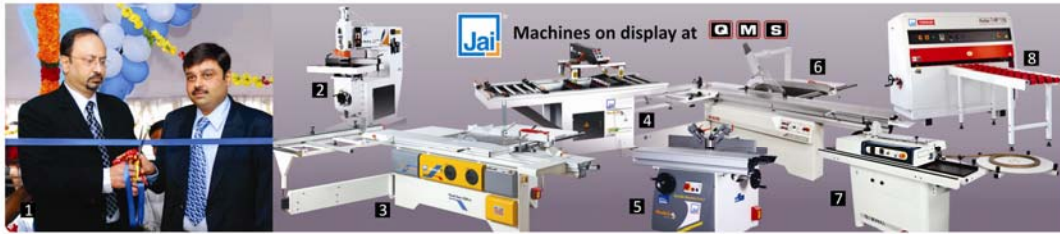
1. Jai Industries directors Nikhil Shah (L), Nirav Shah (R) 2. Hi-speed router 3. Panel saw 4. Double head multi boring 5. Spindle moulder (2 to 5 Modula m/cs.) 6. Scm-Panel saw 7. Scm-Edge bander 8. Turanlar - Throughfeed roller press... and many more.
